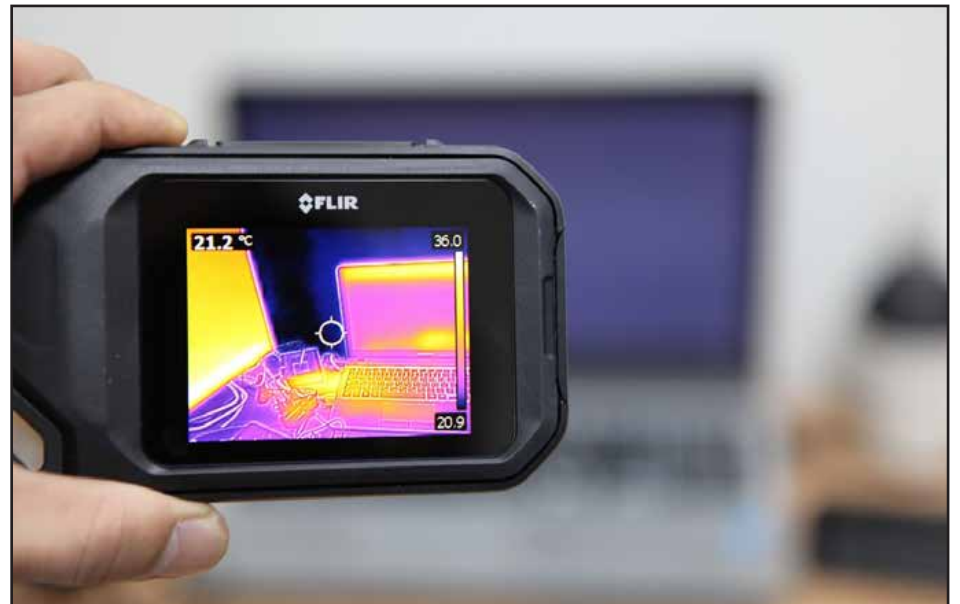
An infrared camera detects heat waves in a similar way to how your eyes detect light. So infrared camera’s can “see” heat. Thermal imaging uses a computer to create a visible image from the invisible heat waves. pic: Pixabay/withplex
