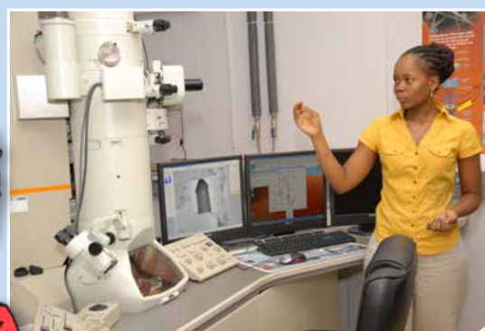
Ms Charity Maepa with a transmission electron microscope used to get information on the inner structure of nanoparticles.
