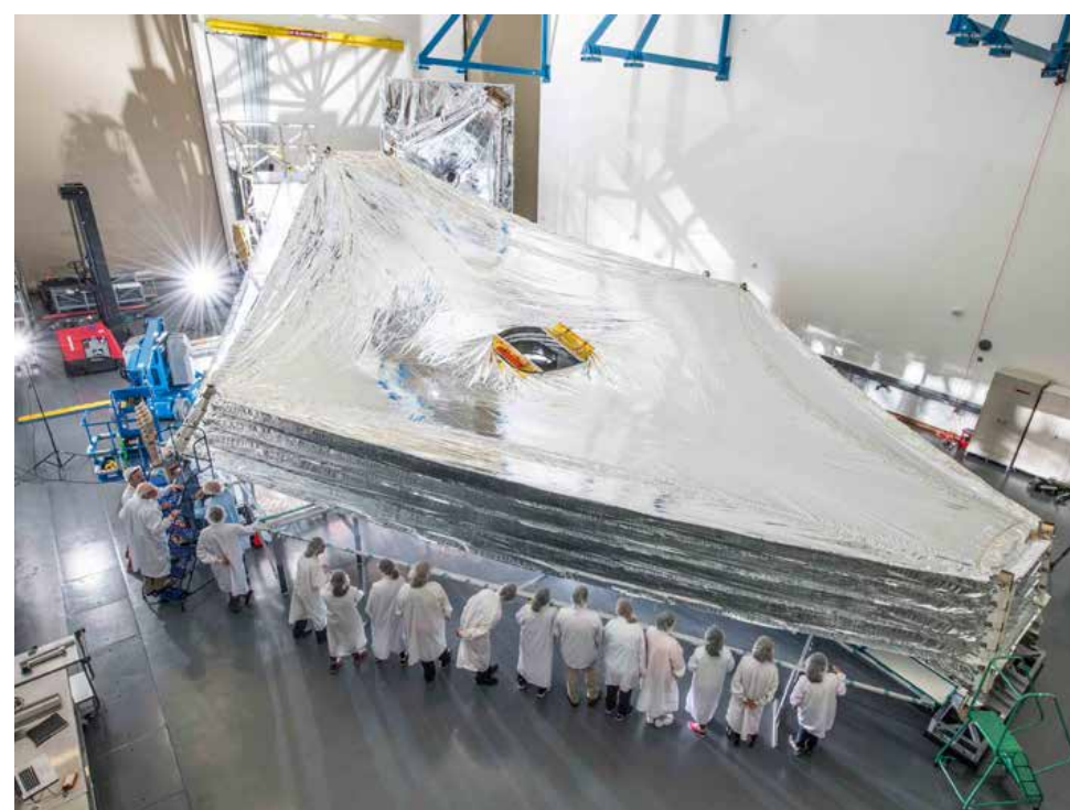
During development, scientists are seen standing around the netball field-sized sunshield designed to keep the JWST extremely cold in order to take the best possible pictures of the universe. Pic: NASA/Chris Gunn
