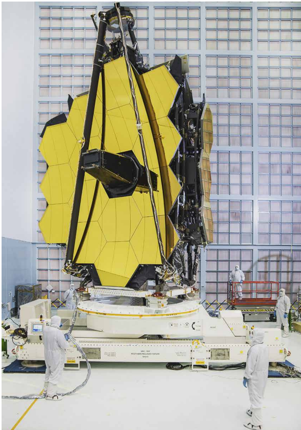
The hexagonal primary mirror of the Webb telescope during production, shown here with two sides folded to fit into the rocket for launch. Pic: NASA/Chris Gunn
